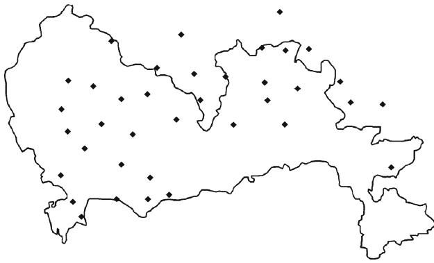
Fig. 4 The distribution of GPS/leveling points in Shenzhen
